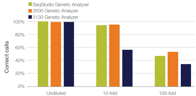
Figure 4. Titration of cell suspensions dried onto NUCLEIC-CARD device. Cell suspensions were prepared at the concentrations shown in the table, then serial dilutions of those suspensions were analyzed using NUCLEIC-CARD devices and the Identifiler Direct kit. The average percentages of correct allele calls across all cell lines at the indicated dilutions are shown.
